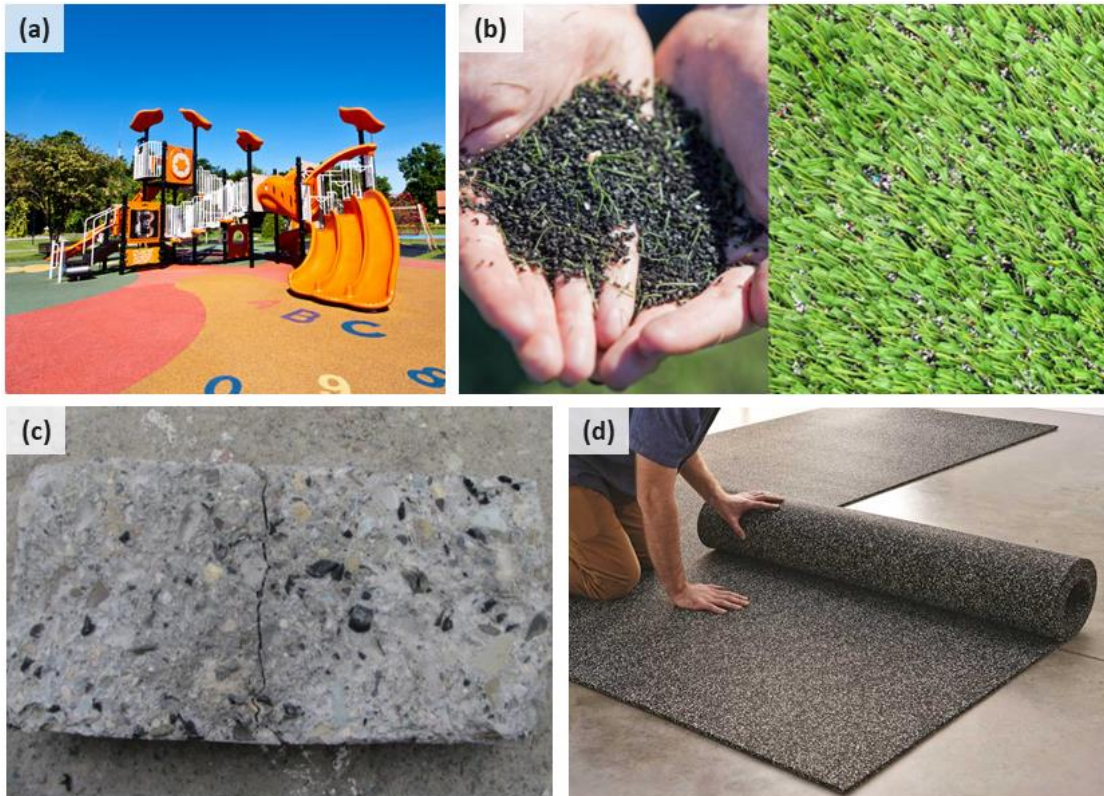
Figure 3.12: Applications for recycled crumb rubber: (a) playgrounds, (b) filling for artificial turf fields, (c) concrete and (d) flooring
