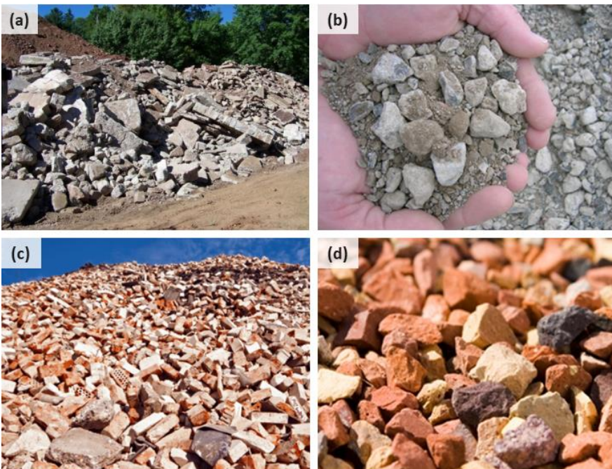
Figure 3.2: Images of (a) reclaimed concrete, (b) crushed concrete, (c) stockpiled brick, and (d) crushed brick
