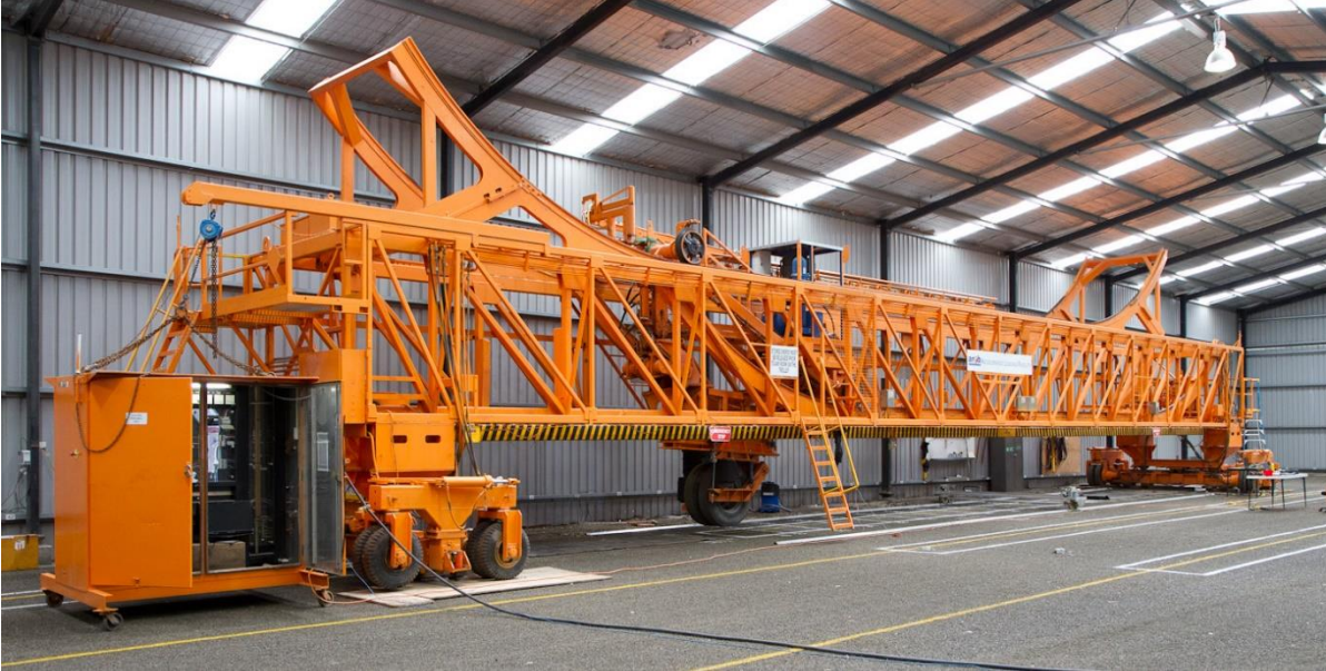
Figure 3.1: The ARRB Accelerated Loading Facility (ALF) has been used extensively to assess the performance of recycled materials in road pavements
